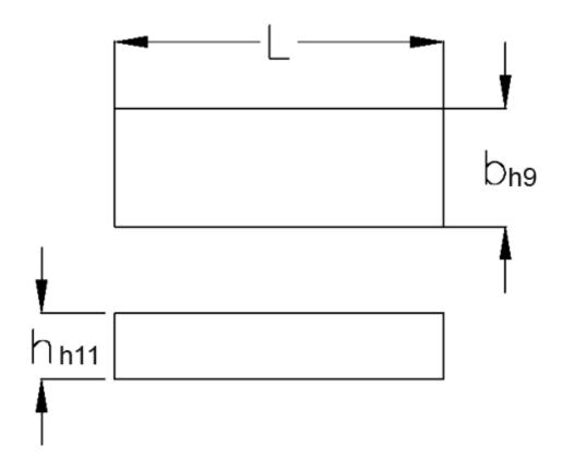
$\begin{array}{ll} b & = 18 \\ h & = 11 \\ L & = 63 \\ Tolerance \ b = 0.043 \\ Tolerance \ h = 0.110 \end{array}$
